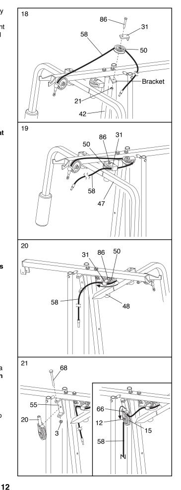
22. See the inset drawing. Attach a 3 1/2" Pulley (15) and a Cable Trap (66) to the upper hole in a Long "U"-Bracket (57) with a 3/8" x 2" Bolt (12) and a 3/8" Nylon Locknut (21). Be sure that the Cable Trap is inside the Long "U"-Bracket. Note: This may come pre-assembled.
